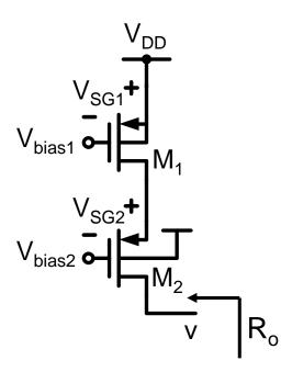
Voltage drop on the two MOSFETs must be minimized to increase voltage swing
