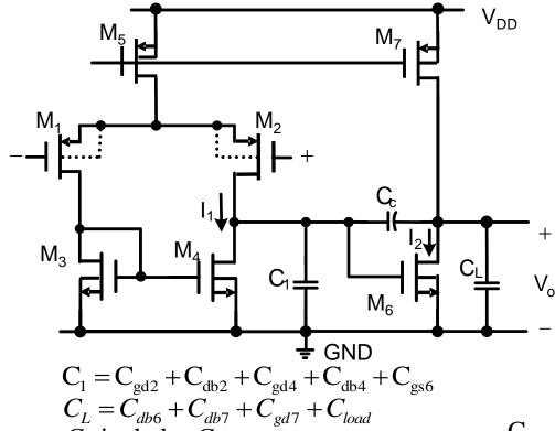
$$C_{1} = C_{gd2} + C_{db2} + C_{gd4} + C_{db4} + C_{gs6}$$
