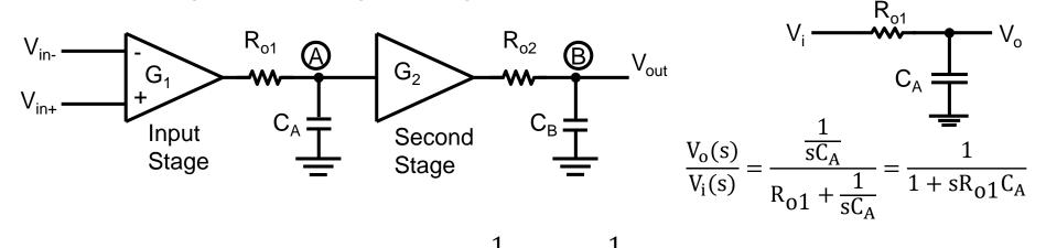
$$A_{V}(s) = \frac{V_{out}(s)}{V_{in}^{+}(s) - V_{in}^{-}(s)} = A_{v}(0) \frac{\frac{1}{sC_{A}}}{R_{o1} + \frac{1}{sC_{A}}} \frac{\frac{1}{sC_{B}}}{R_{o2} + \frac{1}{sC_{B}}} = A_{v}(0) \frac{1}{(1 + \frac{s}{S_{A}})(1 + \frac{s}{S_{B}})}$$
