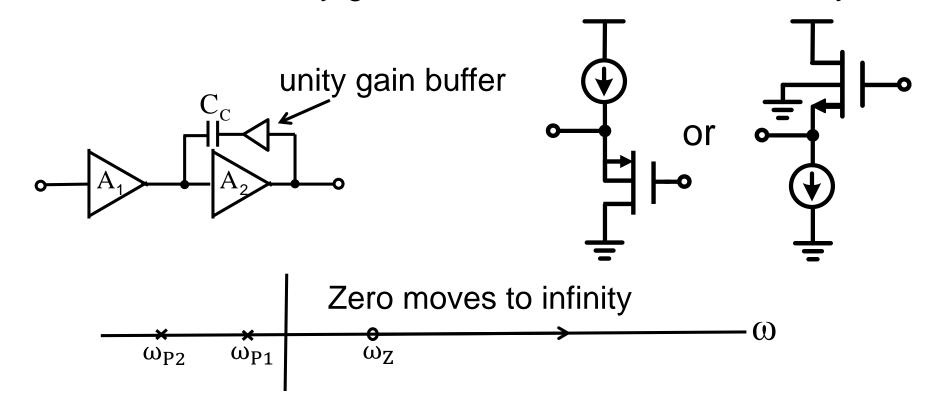
$$A(s) = \frac{A_0}{(1 + \frac{s}{\omega_{P1}})(1 + \frac{s}{\omega_{P2}})} \quad \text{where} \ \ \omega_{P1} \approx -\frac{g_{m1}}{A_0 C_C}, \ \ \omega_{P2} \approx \frac{-g_{m6}}{C_L}$$
