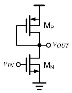
$$\begin{aligned} v_{IN} &= V_{IN} + C \sin \omega t \\ v_{OUT} &= V_{OUT} + AC \sin \omega t \end{aligned}$$
