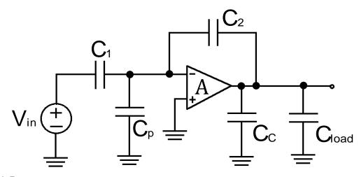
$$\beta = \frac{1/[s(C_{_1} + C_{_p})]}{1/s(C_{_1} + C_{_p}) + 1/sC_{_2}} = \frac{C_{_2}}{C_{_1} + C_{_p} + C_{_2}} \; \; ; \; C_{_P} \; \text{is parasitic capacitance}$$
